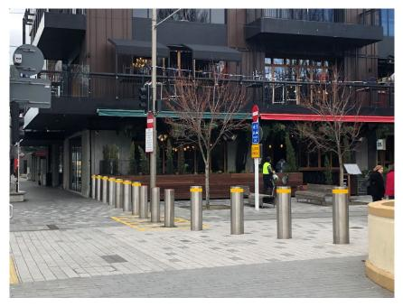
Installed at Oxford Terrace, Christchurch are 11 static bollards and a set of 3 retractable bollards. The retractable bollards are installed across Oxford Terrace, at its junction with Hereford Street, where the tram line is located. The static bollards are positioned surrounding the entrance foot traffic where
